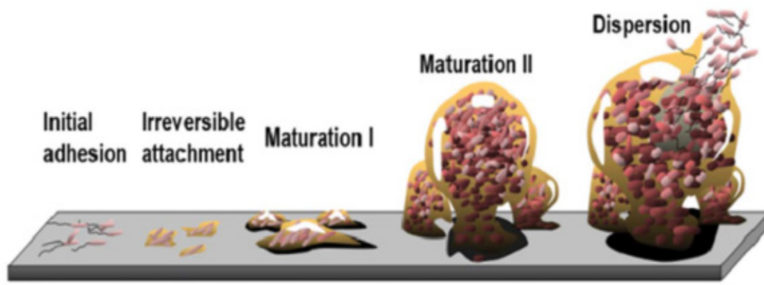
Figure 7: Evolution of biofouling on membrane surface (Zhu et al., 2018)
