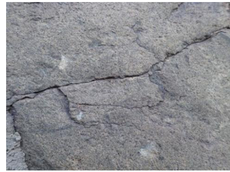
Figure 8 Schematic Diagram Showing Features of Blistering and Splitting
