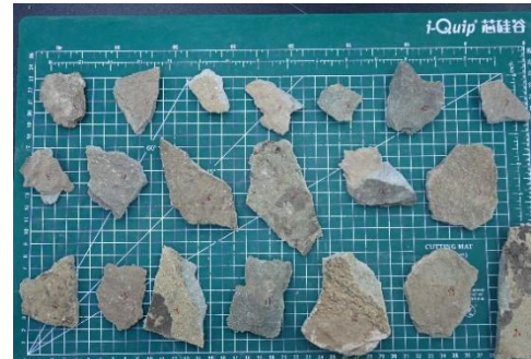
Figure 10 Schematic Diagram of Sheet-Like Detachment Morphology
